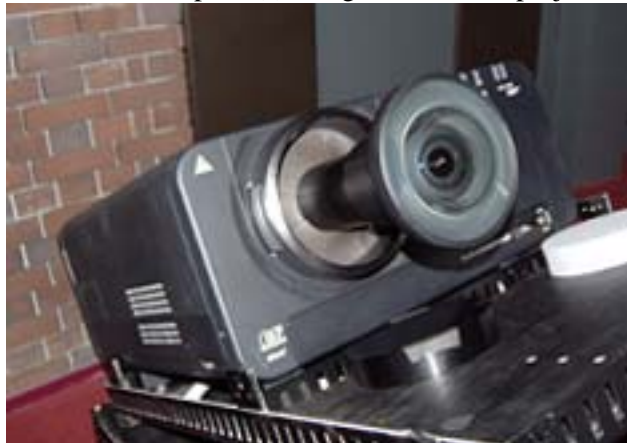
Fig.3. Panasonic DW-10000 projector with Togen circular fish eye lens.
