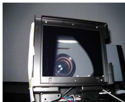
Photo 4. Blending plate installation to projectors
