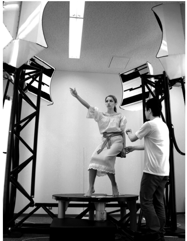
Fig.7. 3D scanning of the shape of an actual person
